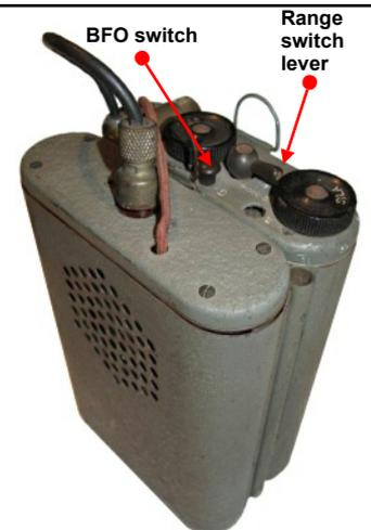
The Polish Stanmore OP-3G receiver was a variation of the OP-3 which had a built-in loudspeaker in the battery compartment (right). It was otherwise a standard OP-3. See also Chapter 24 of WftW Supplement.
